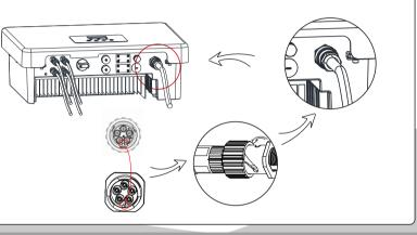
4. Tighten the screw of the back shell and the cable nut.
