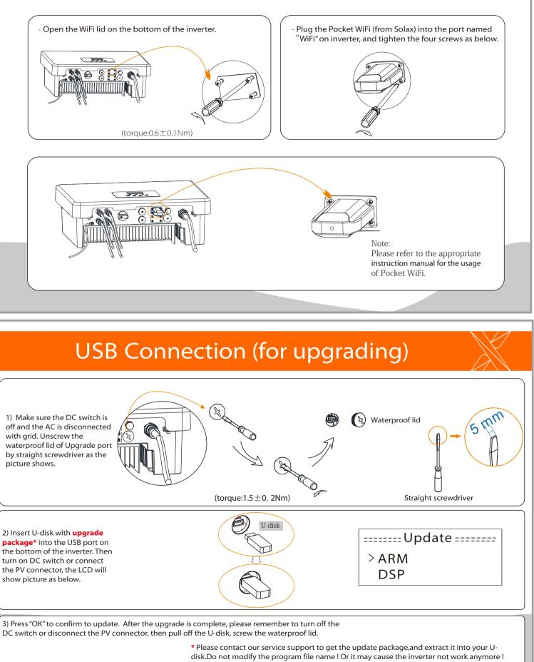
1) Make sure the DC switch is off and the AC is disconnected with grid. Unscrew the waterproof lid of Upgrade port by straight screwdriver as the picture shows.
