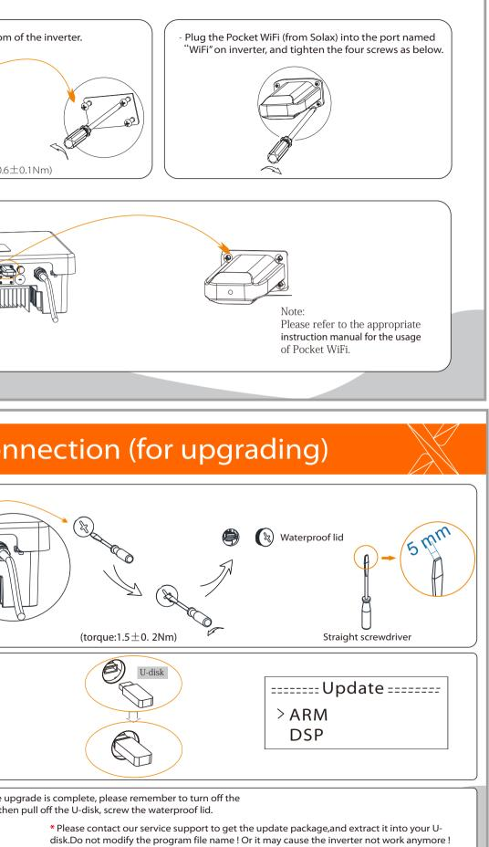
2) Insert U-disk with upgrade **package**\* into the USB port on the bottom of the inverter. Then turn on DC switch or connect the PV connector, the LCD will show picture as below.
