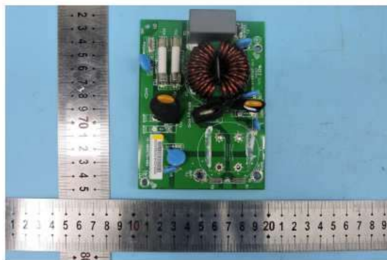
Figure 14 General Appearance of the PCB
